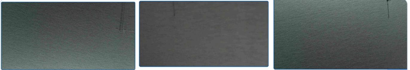
Needle line — for most mills, one of the two most common defects.
